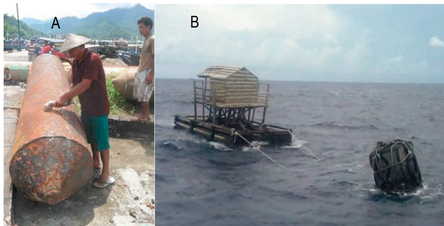
Figure 2. Pontoon (A) and Styrofoam FAD (B)
